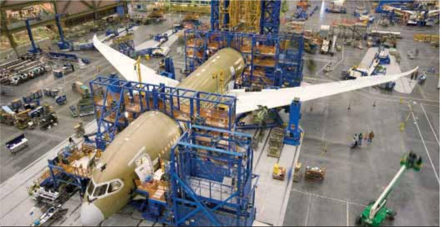
Composite materials make up 50 per cent of the primary structure of the 787 including the fuselage and wing.
