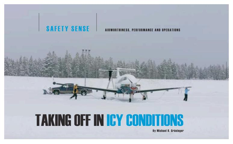
ICE AND FROST FORMATION ON the exposed surfaces of an aircraft poses a serious danger for safe aircraft operation. Even small amounts of clear or rime ice cause a loss of lift, increase in mass and control problems. Ice, snow or frost with a thickness and roughness similar to sandpaper on the leading edge and upper surface of a wing can reduce lift by as much as 30 percent – and increase drag by 40 percent!
