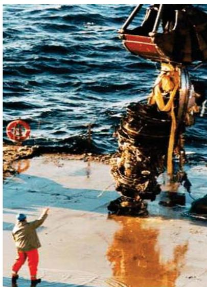
of the last minutes of flight 111 was made difficult by the early failure of the FDR and CVR. Hence the events leading up to the impact with the ocean were reconstructed based on forensic examination of the wreckage fragments.
