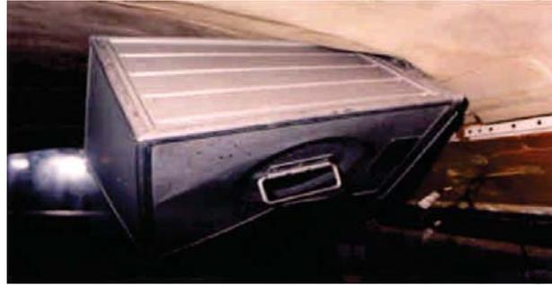
Q” or simply “Arthur” unit adjusts the artificial feel of the elevators according to airspeed and horizontal-stabilizer position.
